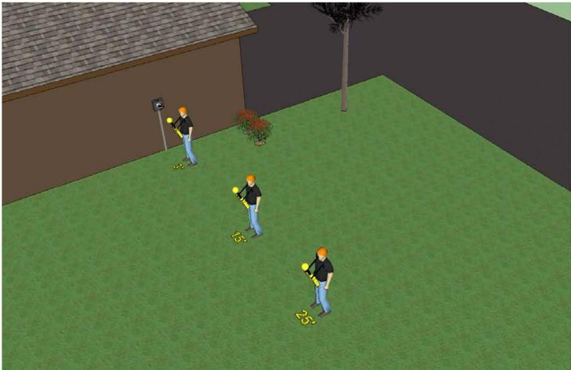
**Figure 2.** Illustration of the measurement of RF fields at different distances, ranging from one foot to 25 feet from the front surface of the smart meter.
