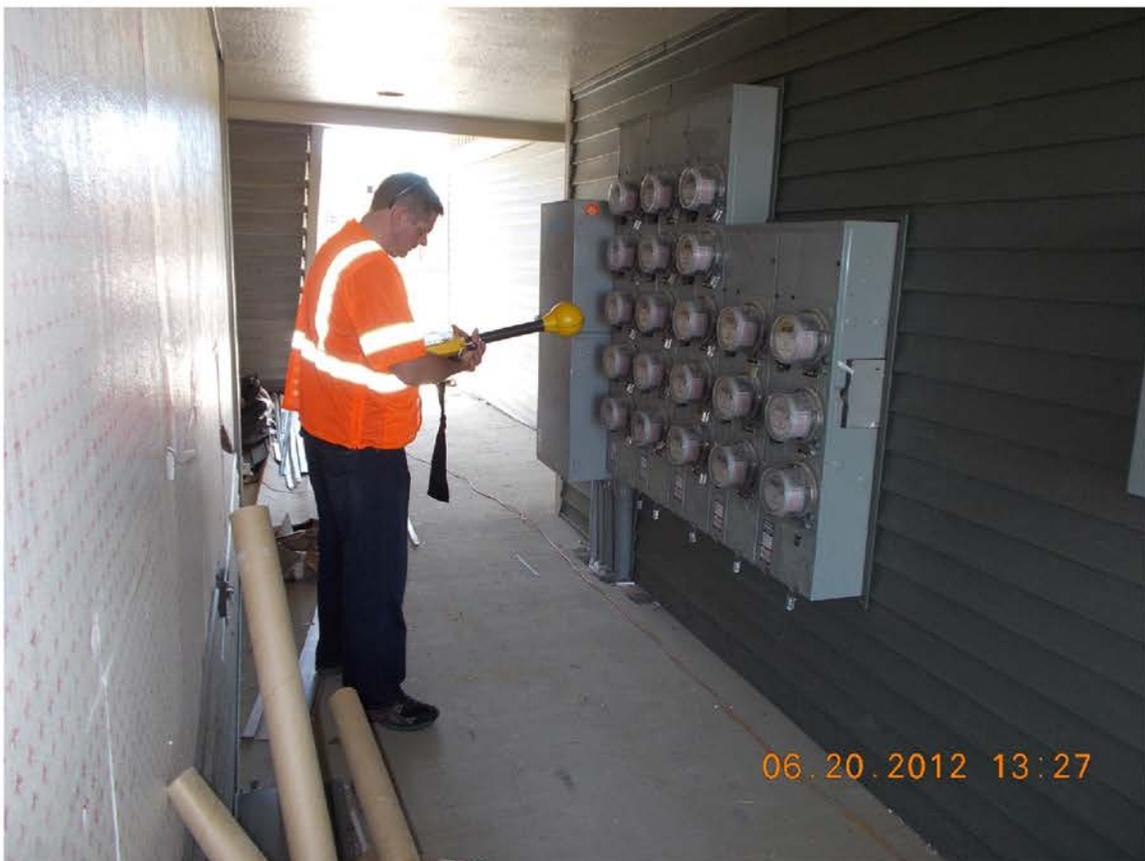
**Figure 6.** Performing RF field measurements in front of a 21 meter bank of smart meters at an apartment complex under construction. Measurements were also performed inside the apartment facing the meter bank and inside the apartment directly behind the bank.
