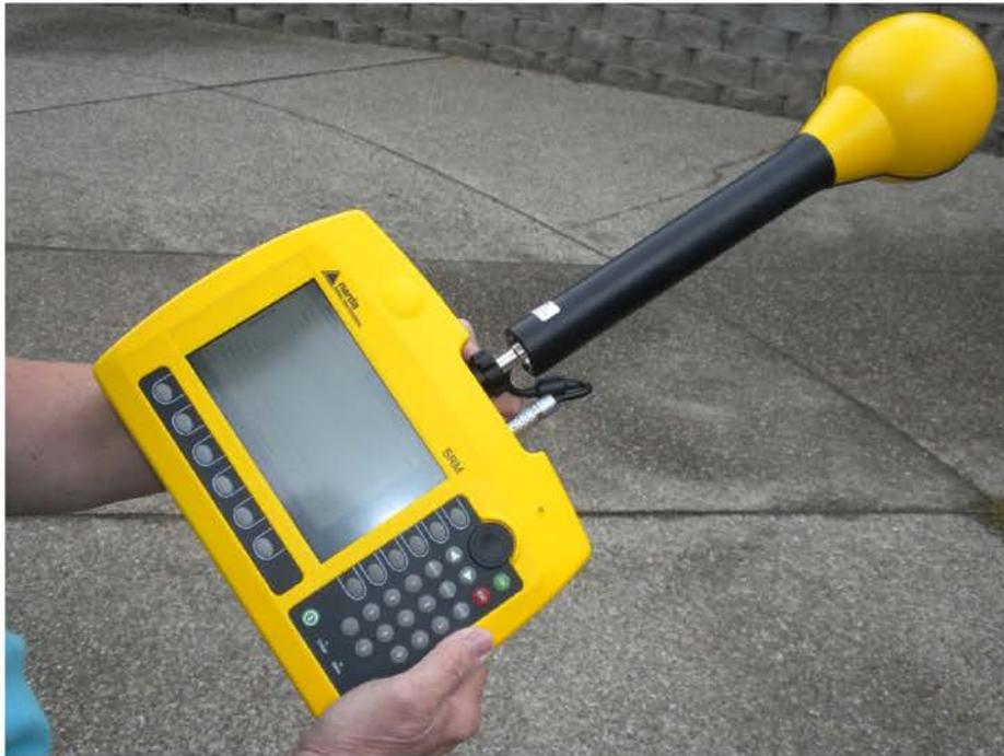
**Figure 3.** The Narda SRM-3006 Selective Radiation Meter is based on Fast Fourier Transform (FFT) spectrum analyzer technology and uses a probe/antenna to measure the absolute magnitude of incident RF fields across the frequency range of 26 MHz to 3,000 MHz and digitally converts the detected field to the equivalent percentage of the FCC MPE.
