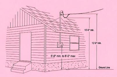
The mast used for attachment of the service drop must be a minimum of a 2-inch rigid steel galvanized conduit, with a suitable attachment to the building to support the weight of the service conductors. Determination of mast height should be made according to applicable service conductor clearances first, then a determination can be made whether mast height will require guying.
